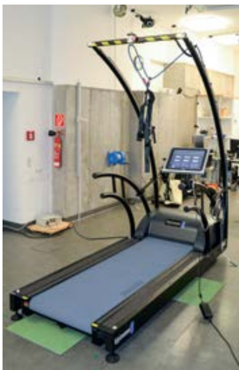
pulsar® 3p with special non reflecting black powder coating, external cables for fast disassembling of handrails for 3D motion analysis at biomechanics department, University of Salzburg, Austria.
