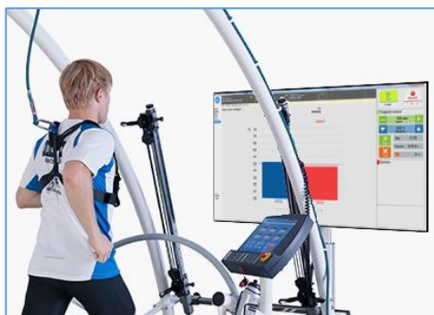
Fig. 4: gait symmetry (left vs. right) loading peak force visualization as an online biofeedback for patient and therapist
