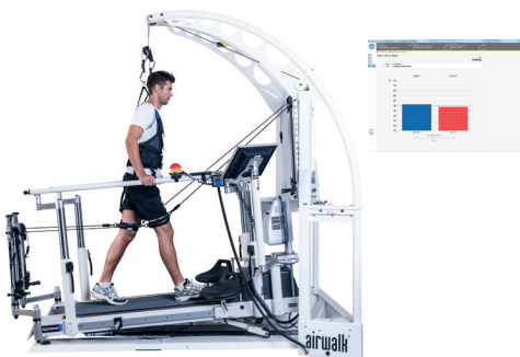
gait symmetry with bio-feedback left vs. right and on-line active gait correction with robowalk
