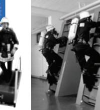
ladder ergometer running machine h/p/cosmos discovery® h/p/cosmos mercury® 150 x 50 cm (59.05" x 19.68") running surface 75° incline 0 ... 40 m/min speed 0 ... 22 km/h (0 ... 13.6 mph) speed
