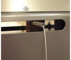
**rope alignment slide** which is guiding the position of the rope.
