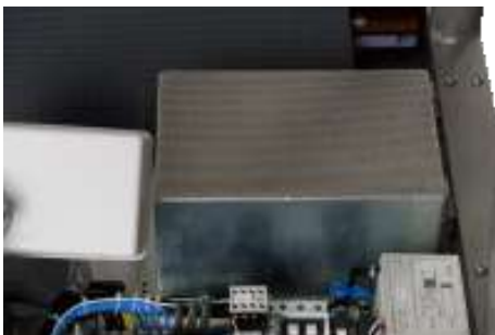
Frequency inverter metal housing (for shielding)
