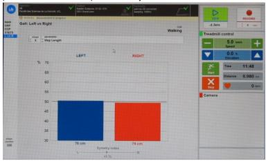
The "Left/Right" screen is used to provide feedback to the operator or to the subject during the exercise. Any parameter can be displayed in a simple left vs right presentation. A symmetry index is also displayed in percentage of the average.
