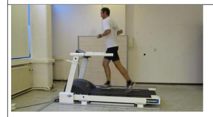
At a higher speed, the gaitway system detects that the subject is now running. The ground reaction forces are also displayed together with the vertical force under each foot. The pattern is now different and also displays a very moderate foot slap for this subject. The scales of the plot can be changed easily by using the mouse wheel.
