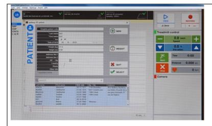
Before recording data we will click in the "Patient" box and select the patient record in the data base. Then, we check the patient body weight using the gaitway system by entering in the "Weighing scale" mode.
