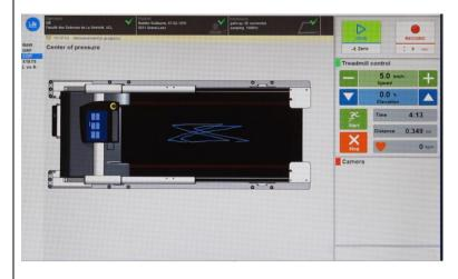
The third panel shows the center of pressure. You can see the butterfly pattern on the treadmill surface and how the system follows the subject as he moves on the locomotion surface.
