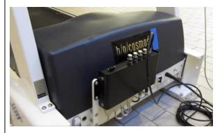
The load cells are mounted to a dedicated frame that is bolted to the floor. This ensures an optimal rigidity and an optimal signal quality. The 3D amplifier mounted at the front delivers the signals to the software via an Ethernet interface.
