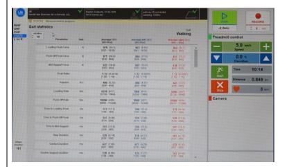
The "Stats" screen shows a number of indices computed for each step. The gaitway system automatically detects the gait. There are time and force parameters and also parameters relative to the position of the center or pressure. The parameter values are computed on the fly for the selected number of strides.
