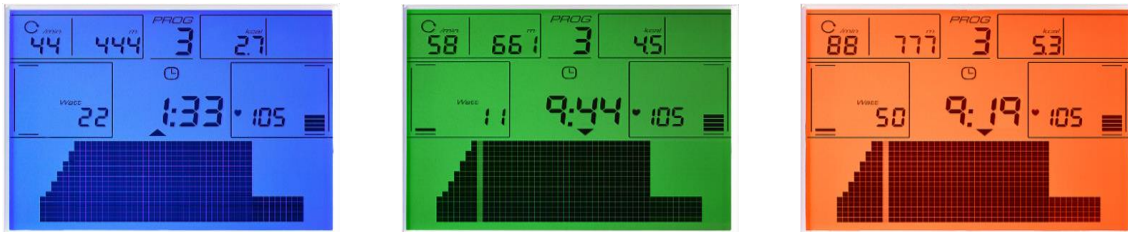
Fig.4: Multicolor backlight function for a visual indication of workout target.
