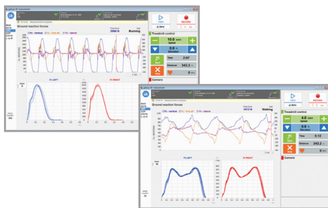
3 component force measurement, F_z , F_y , F_x during running (left) and walking (right) on the gaitway® 3d
