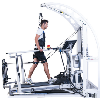
gait symmetry with bio-feedback left vs. right and on-line active gait correction with robowalk
