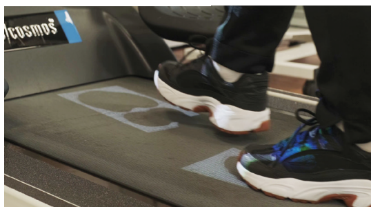
adaptive visual cueing [cos101291-01] with projected steps on the treadmill belt
