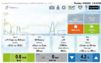
The MCU6 summary screen shows all relevant data of the workout including average and max. speed, elevation, duration and heart rate as well as biomechanical indicators such as steplengths and cadence.
