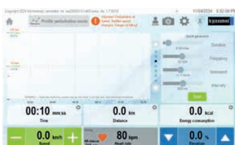
UserTerminal MCU6 featuring a quick generator module for fast and easy perturbation setup and several tests (e.g. Stroop test)
