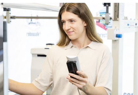
Therapist using the system for manual gait therapy, manually adjusting the speed and elevation with the additional keyboard [cos104551].
