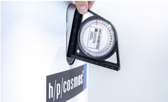
The exact inclination of the camera has to be transferred to the software using the supplied inclinometer.
