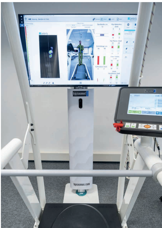
Live view and tracking of the subject on a mercury® med treadmill
